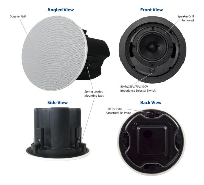
The **Ceiling Speaker** (CS-70V) has a tuned ported enclosure that provides superior bass response while maintaining efficiency. The speaker grill comes pre-installed from factory. An impedance selector switch is easily accessible under the removable grill. Spring-loaded mounting tabs make for easy and secure installation. All metal, spring-loaded terminals provide easy and convenient attachment of speaker wires. Metal speaker back meets UL 2043 criteria for plenum installation.
