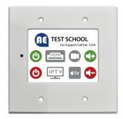
The AV Touch Wall Control (ITC-1) is a programmable 3.5" wall panel for use with controllable amplifiers, such as the GL-300 or MS-450. The digital interface gives installers the flexibility to customize the buttons in each classroom to be perfectly suited for any compatible devices in the room. Teachers can then use the one-touch buttons to power on or off any connected device.
