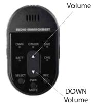
A momentary press of the PWR button will mute or unmute the microphone audio. If muted for more than 5 minutes, the microphone will turn off automatically. Step 1. Connect the micro-USB plug of the charger to the DC input terminal of the microphone.
