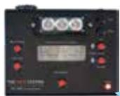
LCD should display “Status OK” and “Netwk OK”. If not, check the network cable connection between this box and the network connection plate on the wall or floor. Contact your Network Administrator or IT department if you cannot resolve the problem.
