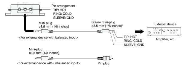
\* Cable with optimal plug type should be selected depending on the device to be connected.
