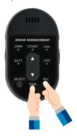
**3.** Successful microphone linking will produce a *beep* through the system, and the *BATT* LED on the microphone will glow green.
