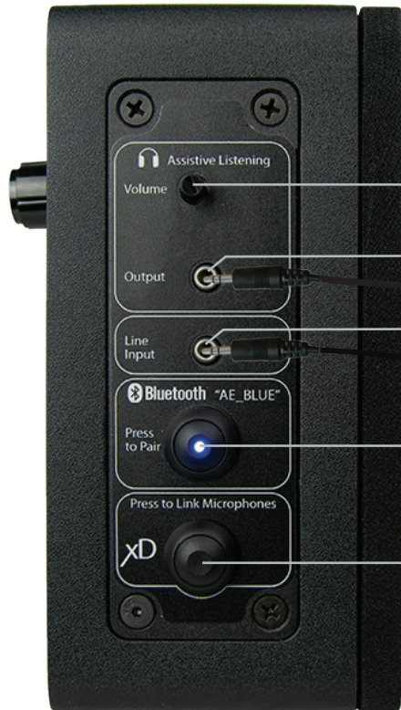
Side Panel Connections (Left end—viewed from the front)
