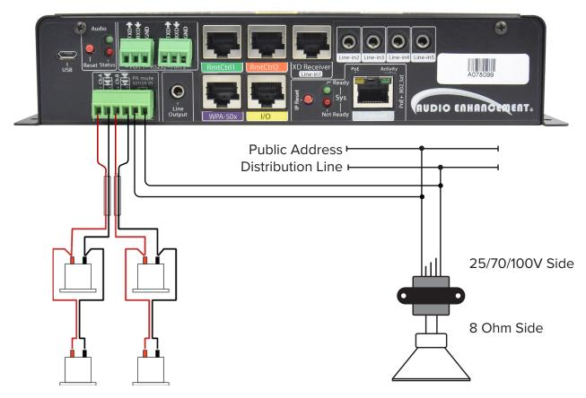
When using 4 speakers, wire ceiling speakers parallel in the ceiling—bringing one speaker wire per pair to the MS-300 amplifier channel.
