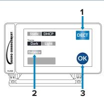
The pairing process is done through the configuration screen. To access the configuration screen, press the corners of the screen in the order shown above.
