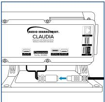
Locate the USB-C input on the back of the CLAUDIA device and plug in the supplied USB-C Power Supply.
