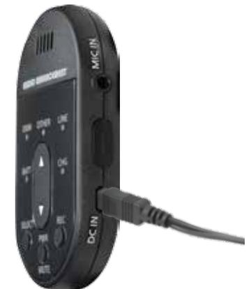
Press and hold the PWR button to turn the microphone on or off.
