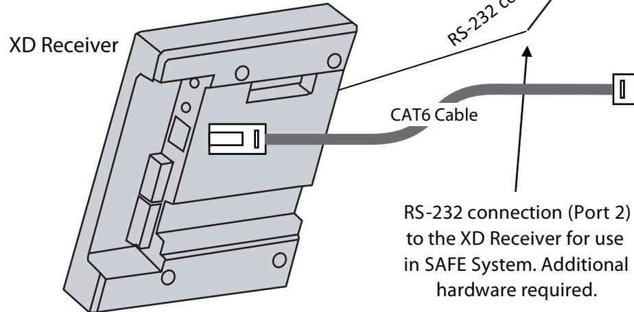
RS-232 connection (Port 2) to the XD Receiver for use in SAFE System. Additional hardware required.
