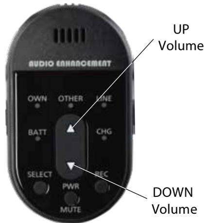
Note: Volume levels on line inputs can only be adjusted via USB. Install and run the GL-300 software before connecting the USB.
