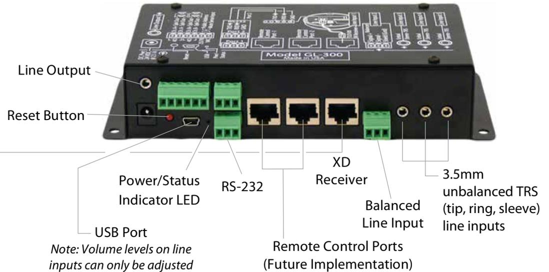
Note: Individual volume levels of the Teacher Microphone can be adjusted with the UP and DOWN volume buttons. Input on the GL-300 can be controlled via USB which is mic1, mic2, and Line mixed audio.
