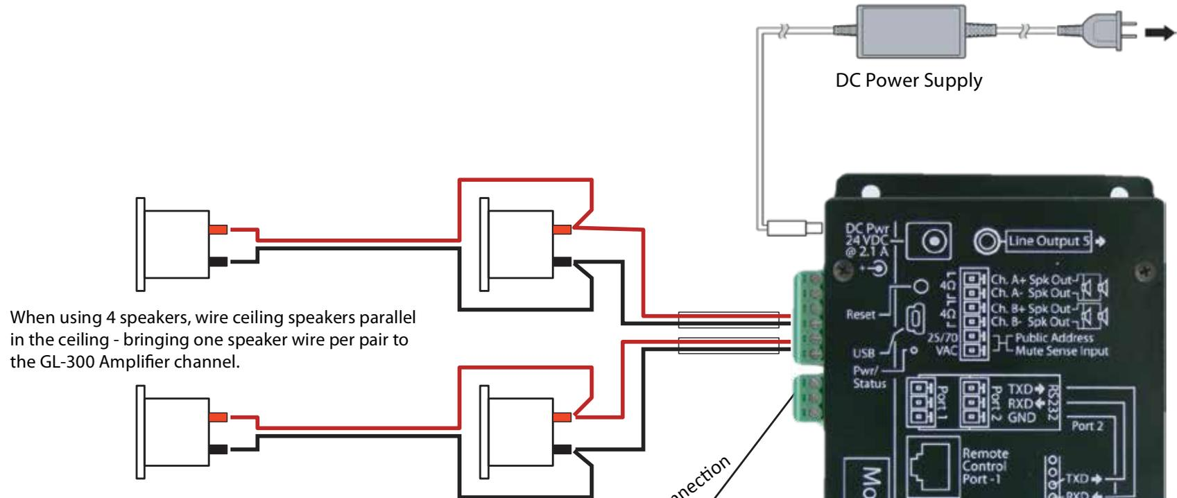
When using 4 speakers, wire ceiling speakers parallel in the ceiling - bringing one speaker wire per pair to the GL-300 Amplifier channel.
