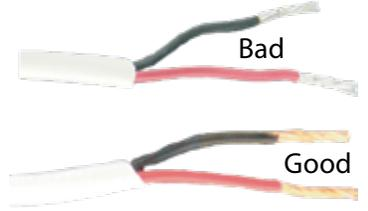
Use a set of tin leads and connect to the speaker. Then cut the speaker wires to appropriate length. Strip the newly cut ends to bare copper before inserting into the screw compression
