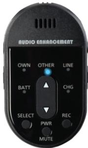
To adjust the Student Microphone (**OTHER**) volume, first press the **SELECT** button so that the LED over the **OTHER** label comes on. Now press the UP/DOWN buttons to control the level of the **OTHER** microphone, which is typically the Student Microphone.
