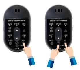
**3.** Successful microphone linking will produce a *beep* through the system, and on the front of the amplifier you will see an additional green LED.
