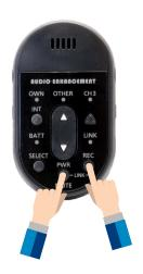
**3.** Successful microphone linking will produce a *beep* through the system, and on the front of the amplifier you will see an additional *green* LED.
