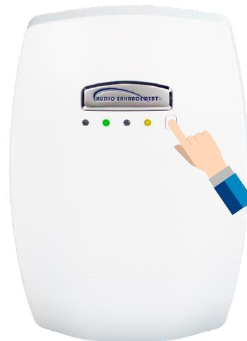
3. With the XD Clear Bridge connected to a USB port on the computer, press the *Link* button on the back of the unit. The XD Clear Bridge LED will slowly blink Green when plugged into a USB Port. After the *Link* button is pressed the XD Clear Bridge will quickly blink green until the link is completed.
