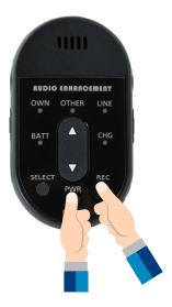
**3.** Successful microphone linking will produce a *beep* through the system, and on the front of the amplifier you will see an additional *green* LED
